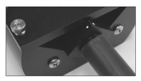
For best repeatability it is important to insert collectors in a consistent orientation. To facilitate this, collectors may have a pair of white dots marked on them. These dots should always be facing up, that is, toward the flat top plate, as shown in Figure 5.
