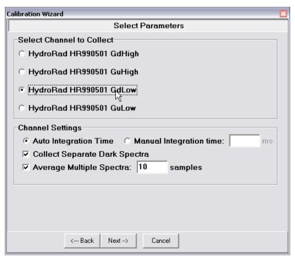
• Check that the SLS "Stable" light is still on, and that the optical head is properly connected to the light collector to be tested. If so, check the appropriate boxes in the dialog box and click **Next**. This will initiate data collection. Note that the data collection time depends on the sensitivity of the HydroRad channel under test. Instruments set up for direct solar illumination may require several seconds for each of the 10 integrations.
