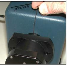
Figure 7 Mounting on a Labsphere port
